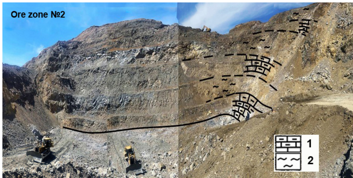
Figure 2.29: Chuluut Tsagaan Del fluorite mine, ore body 2 (photo by Tumenbayar.B, 2023). 1 Fluorite bearing limestone, 2. Metamorphic rock.
