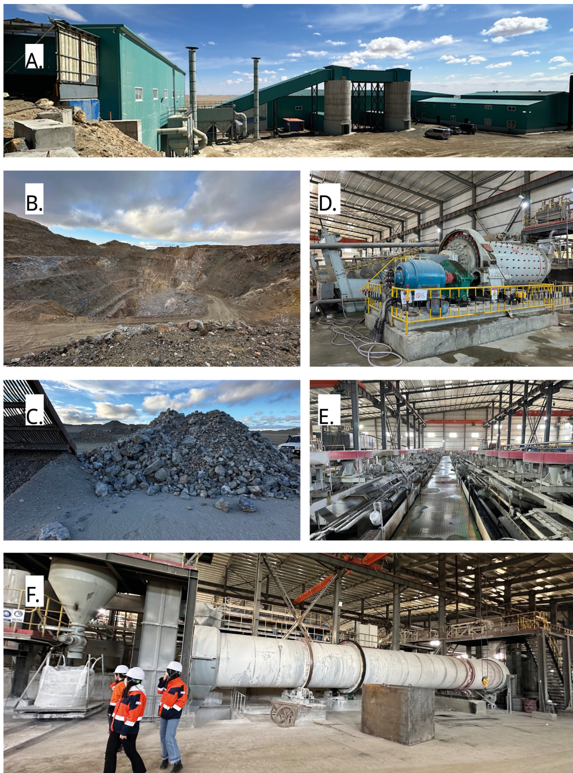
Figure 4.4: GMIT Project team visited Mongol Czech Metal's fluorspar (CaF 2 ) ore beneficiation plant (A.), open pit mine (B.), hand sorted fluorspar (C.), milling section (D.), flotation section (E.) and concentrate drying kiln (F.) (Photos: GMIT).
