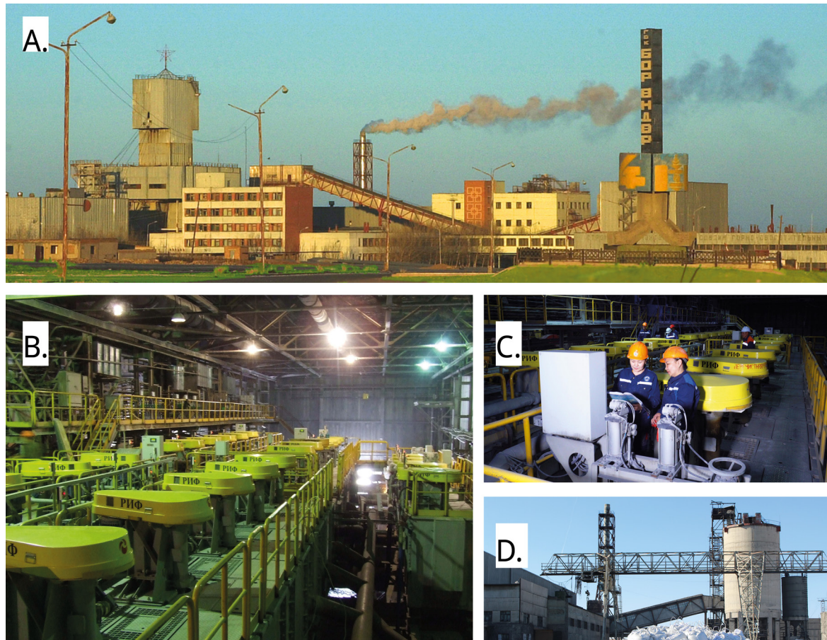
Figure 4.2: \text{CaF}_2 concentrate production plant (A), flotation cells (B,C) and packaged concentrates (D).
