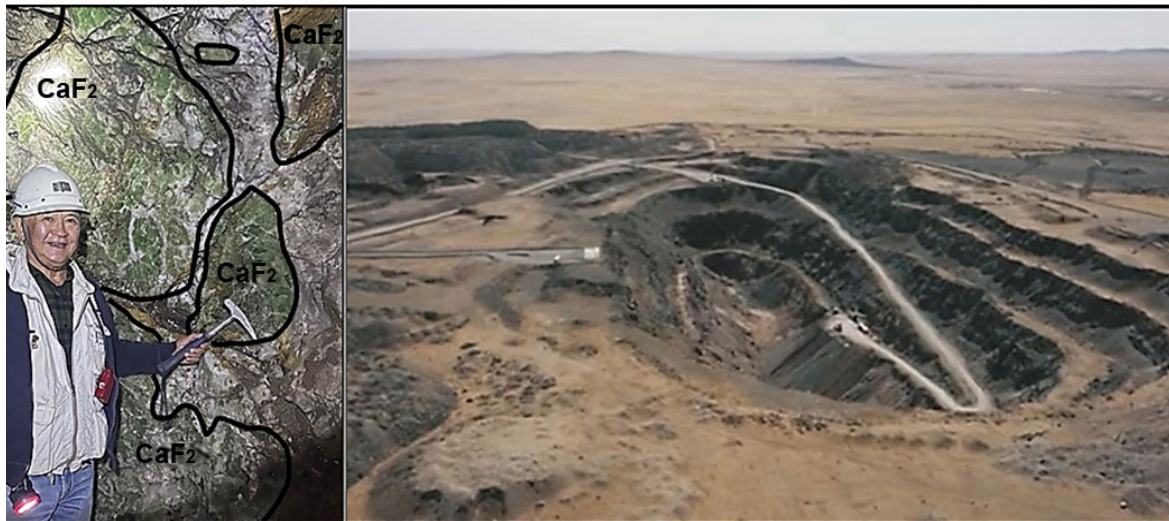
Figure 2.21: Zuun Tsagaan Del mine, 70-meter depth, 65% \text{CaF}_2 , 14 meters thick ore body 7 (Photo by Buyanbal, May 2024).
